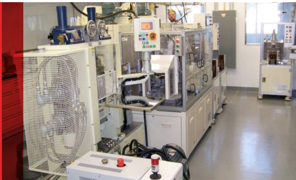
Cell production equipment in dry room
