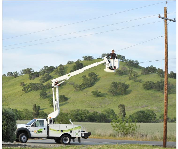
Hybrid utility truck allows for work on utility lines without engine idling. *Photo credit: Altec, Inc.*
