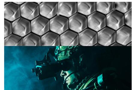
3D printing of microchannel plates such as above with 300 nm walls, enables improved performance at a fraction of the cost. Such plates are key components of advanced performance detectors such as those used in night vision goggles.
