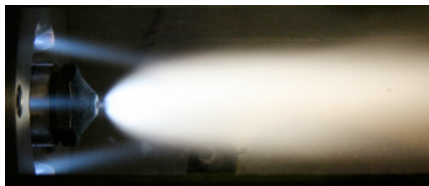
The most advanced diagnostic system for flame spray pyrolysis enables the manufacturing of complex, catalysts in high volumes.
