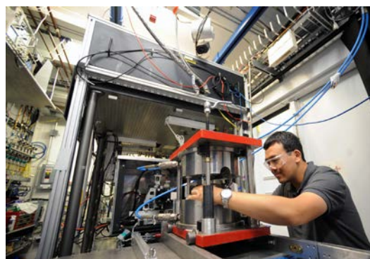
Postdoctoral researcher Feng Shi setting up a sample for an acoustic emission high-pressure and temperature experiment at the APS.
