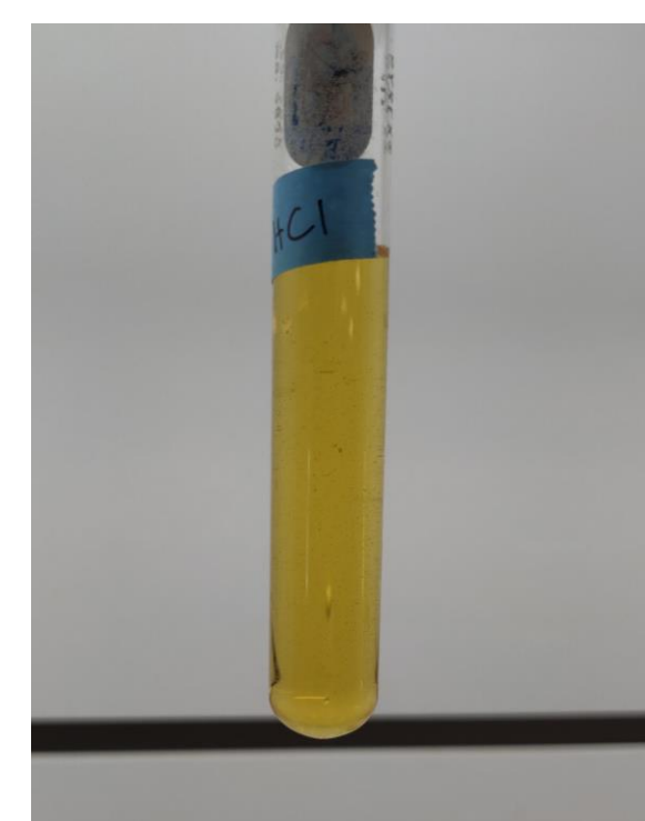
Figure 2: Solution of factory-treated wood and HCl after the addition of KI, forming Lugol's Iodine
