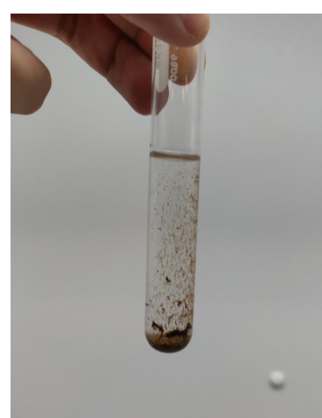
Figure 3: Solution of factory-treated wood and HCl after the addition of \text{Na}_2\text{S} , forming CuS precipitate
