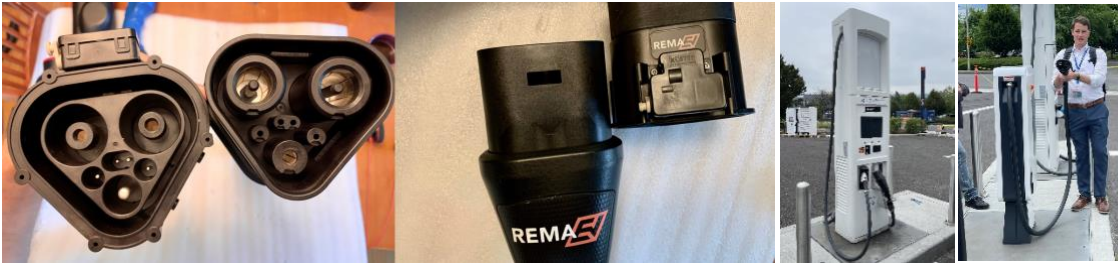
Left to right, preproduction plug and vehicle inlet from Rema. MCS-equipped EVSE at Electric Island Portland, Oregon. (Photos: Ted Bohn, ANL)
