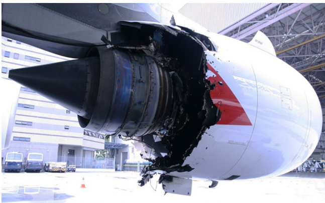
Figure 7.3 Left: In 2010, an Airbus A380 sustained an uncontained engine rotor failure (UERF) of the No. 2 engine as it departed from Singapore while climbing through 7,000 ft. Debris from the UERF hit the aircraft, which led to significant structural damage. Bottom: The culprit was caused by metal fatigue in an oil feed stub pipe due to a slightly misaligned machining that left the pipe a little thinner on one side. [Australian Transport Safety Bureau Investigation #: A0-2010-089]
