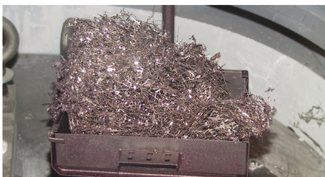
Uranium product collected during advanced refiner testing.
