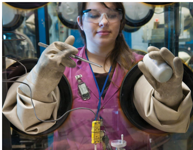
Recovering samples from pyroprocessing testing for analysis.
